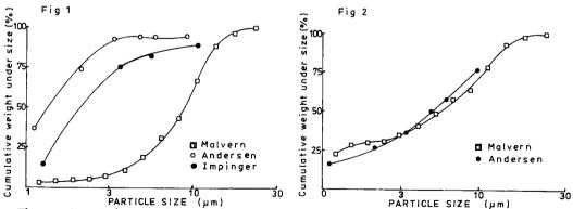
The contrast in results of the aqueous aerosols may be due to evaporation and re-entrainment of smaller particles in cascade impaction on dry plates as demonstrated in the latter experiments. The Malvern 2600HSD instantaneously sizes the aerosol clouds at a short distance (lcm) from the mouthpiece. Since aerosols are directly inhaled from the nebulised system, the Laser diffraction technique therefore provides more realistic particle size measurements for nebulised aqueous solutions.
